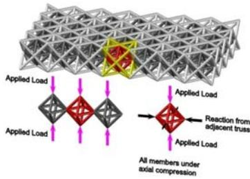
OTEC provides strength and stiffness using a fraction of the material. Compression tests show OTEC approaches the ideal strength-to-weight ratio for bending-dominated lattices at low densities, and in flexural tests OTEC achieves equivalent strength of a solid concrete beam and higher ductility using only 52% of the material.
