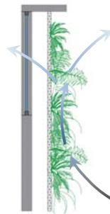
Green facades can provide significant air purification, improving the environment both inside and outside the building. Adding a second façade layer can also provide the thermal benefits of a double-skinned façade system without replacing the entire wall.
