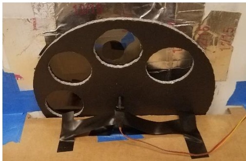
Four-state façade with selectable transmittance of 100%, 80%, 40% & 20% (step motor is also shown)
