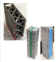
Double-skinned façade (DSF) panels can be constructed using OTEC or 3D printed polymer lattices. These use a fraction of the material of a conventional concrete wall and reduce the thermal transmittance. Conventional concrete DSF panels have been shown to reduce thermal transmittance by up to 43.2%
