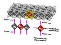
OTEC provides strength and stiffness using a fraction of the material. Compression tests show OTEC approaches the ideal strength-toweight ratio for bending-dominated lattices at low densities, and in flexural tests OTEC achieves equivalent strength of a solid concrete beam and higher ductility using only 52% of the material.
