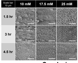
□ The important parameters for our ZnO nanoporous structure are synthesis temperature, solution molar concentration, and synthesis time.
