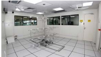
Measurement tree during tests in the double fan room
