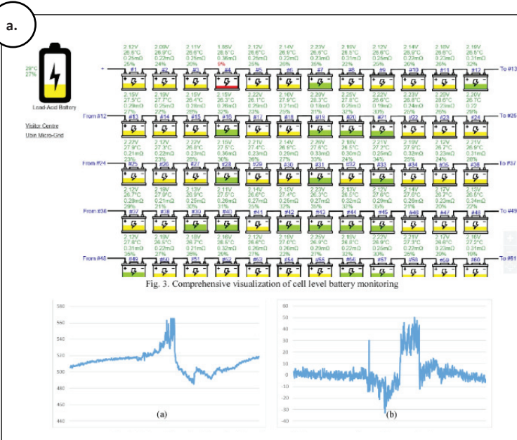
(a.) Cell level monitoring for battery bank (b.) Module level monitoring for PV system.
