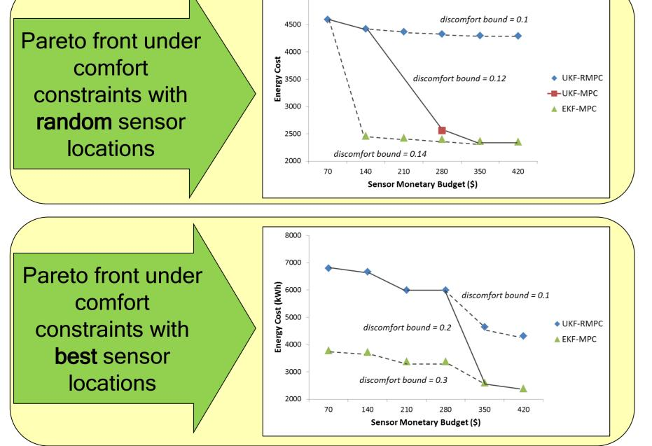
explores the control algorithm design and the sensing platform design together, by analyzing their inter-dependencies through the sensing accuracy.
