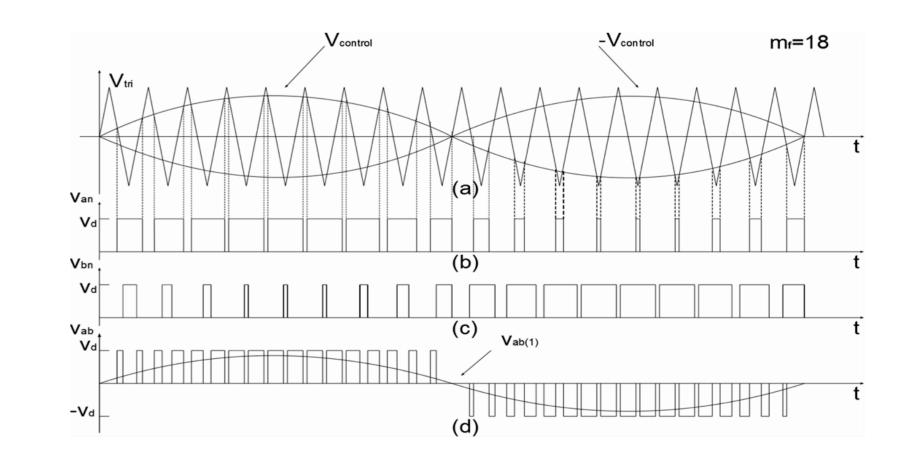
SPWM stands for sinusoidal pulse width modulation. It is a normal PWM wave that has a sinusoidal pulse width.
