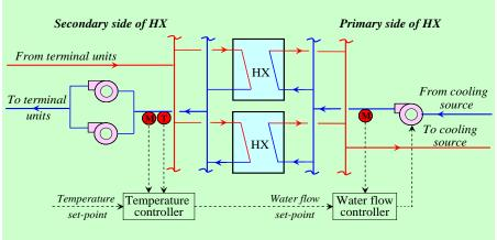
Revised strategy – cascade controller without using any modulating valve
